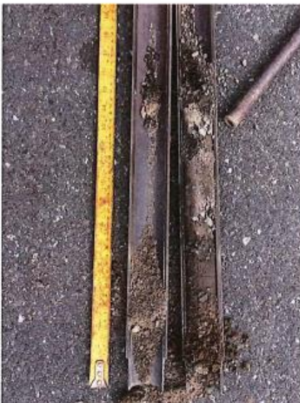
Photo 18 – BH-5, SPT-1 at 0.6 to 1.2m depth showing silty sand and gravel over silt/clay (Photo April 11, 2016)
