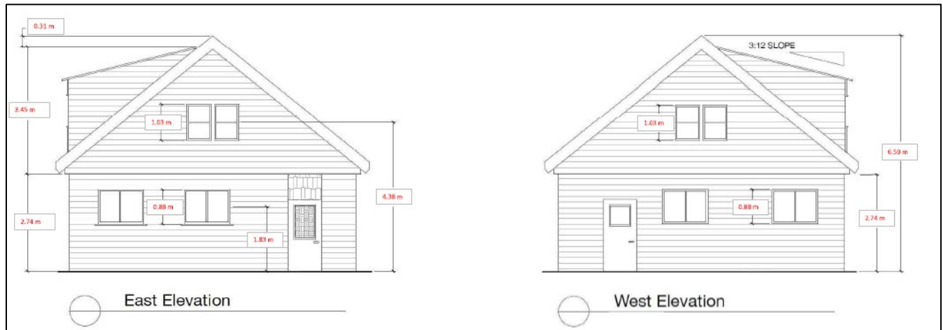
Figure 2. Building elevations. Note that building height for gable roofs is measured from the average distance between the ridge of the roof and eaves.
