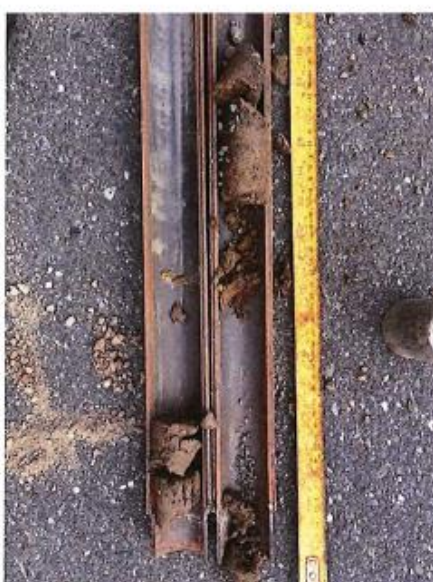
Photo 19 – BH-5, SPT-2 at 2.1 to 2.45m depth showing sandy silt/clay (Photo April 11, 2016)
